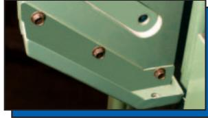
**Note:** *Die doors are* designed to be a point-of-operation barrier and are not intended to stop projectiles.
