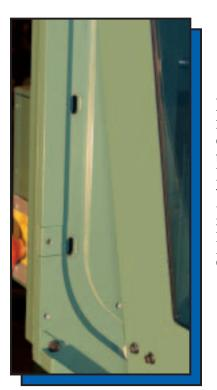
Mounting plates include a machined channel that guides the Delrin® rollers. Holes are located within the channel providing a means for the safety pins to positively lock the door in place.
