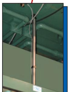
The Pax Die Door Air Assist Option includes a single air cylinder which is operated by a selector switch to raise and lower the door. By utilizing the counter balance weights in conjunction with the air cylinder, minimal air pressure is required to operate the door. This translates into a safer and less complicated design. The Air Assist Option may be required for larger presses or applications that have a reach height that prevents the door from being completely opened manually.
