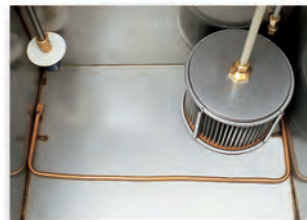
Low Level Float, Air Agitation and Screen Filter
