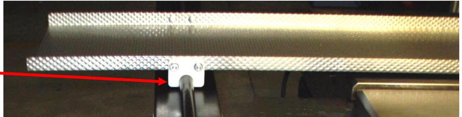
Tray brackets simply snap in place over the round portion of the cross bar without use of tools. The machined, acetal brackets bolt to the side of the conveyor tray and are able to rotate on the cross bar in the event that the tray needs to run on a slight angle.
