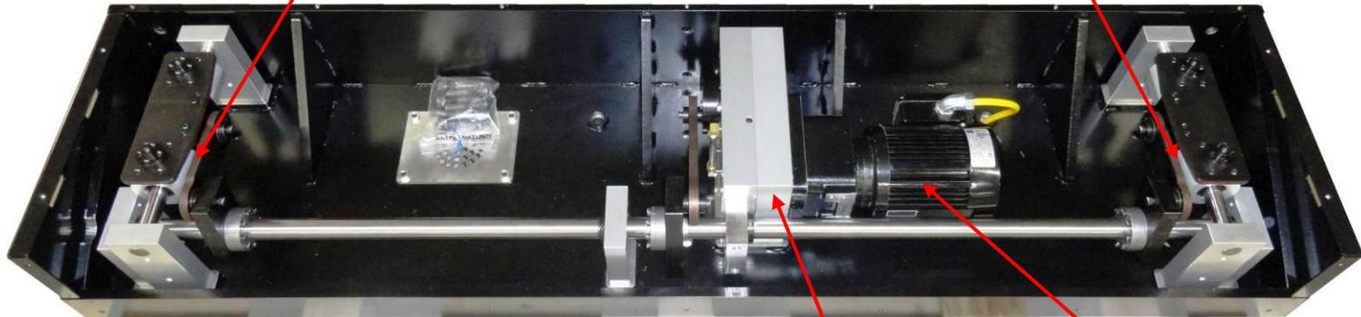
**Elliptical Gear Drive in Sealed Oil Bath**
